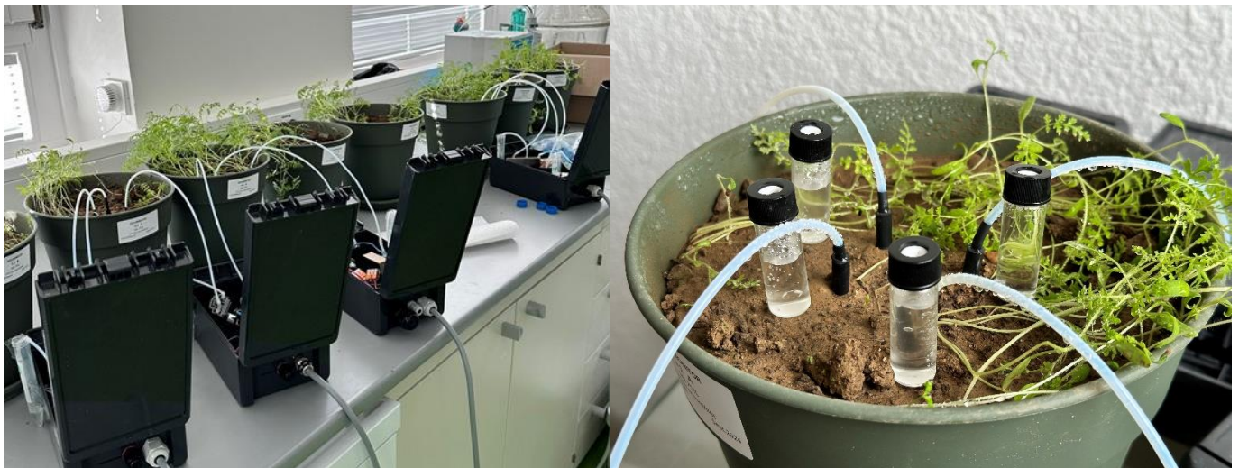
Figure 6: Soil-solution extraction setup; testing the impact of different soil types (left); testing the impact of different sensors (right). Pots contain different soil compositions, as well as fertilization levels, with Phacelia tanacetifolia growing in the pots.
