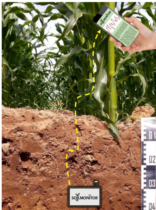
Figure 2: The sensor data will be transferred via LoRaWAN directly or through a repeater into the hands of the farmer.
